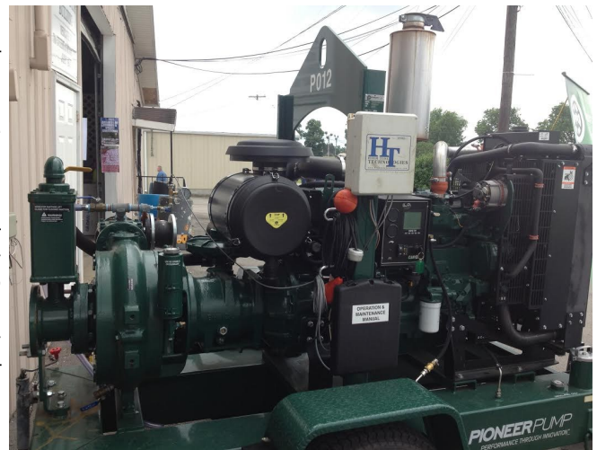
Pioneer pump (PP64S17) fitted with High Tide Telemetry
