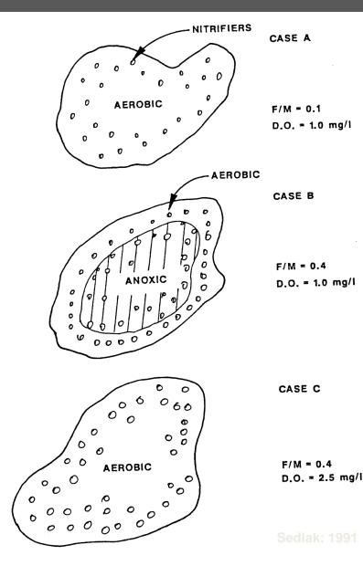
The 3-D Floc concept allows for changes in **ORP** demand due to load or floc condition. Nitirification rates with the same dissolved oxygen vary due to floc.
