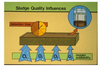
Quantify through comparison of solids weight and volume or space occupied during settling test.
